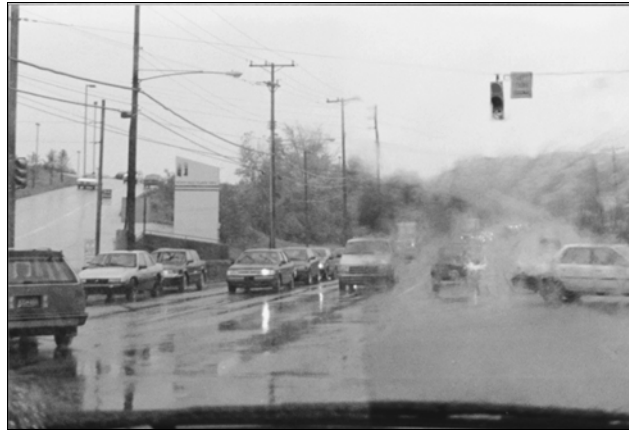
The left side of this windshield has been treated with Aquapel and is much clearer than the right side.
